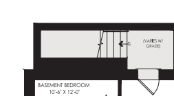
PARTIAL OPT. FINISHED BASEMENT PLAN W/ BASEMENT BEDROOM & BATHROOM FOR WALK- UP BASEMENT
